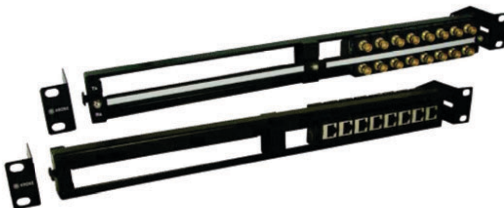
Modular Balun Panel, 75/120 Ohm, 2-8Mbit/s, E1 & E2, Shielded 19" 1RU, 16x1.6/5.6 (f) to 8xRJ45 (f)
