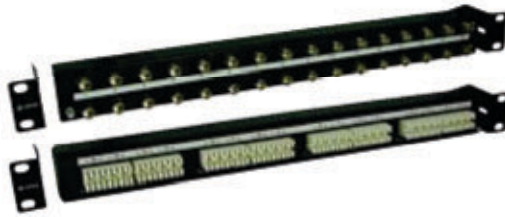
Balun Panel, 1RU, 32xBNC(F) to 8x4Way KRONE Modules, reversible, 2-8Mbit/s Application, 75/120 Ohm, 16xE1 Channels
